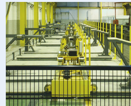
Four computer-controlled manipulators lift, move and position the rails during the forging process.
